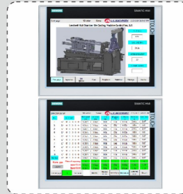
Professional HMI Siemens 9" or 12" Touch LCD and SPC function
