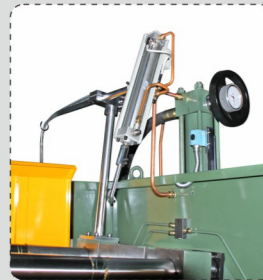
Pneumatic Sweeper for casting removal
